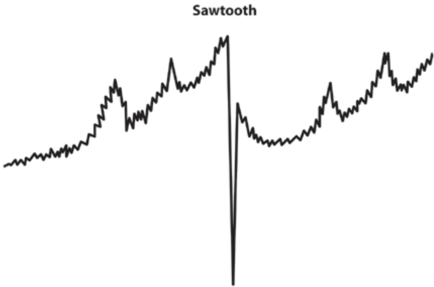
Figure 30 The Sawtooth Waveform is Ideal for Delivering Bunches of Frequencies Simultaneously
